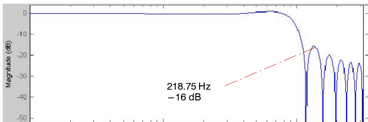
Figure 1.80: Frequency response (all frequencies up to Nyquist frequency)
