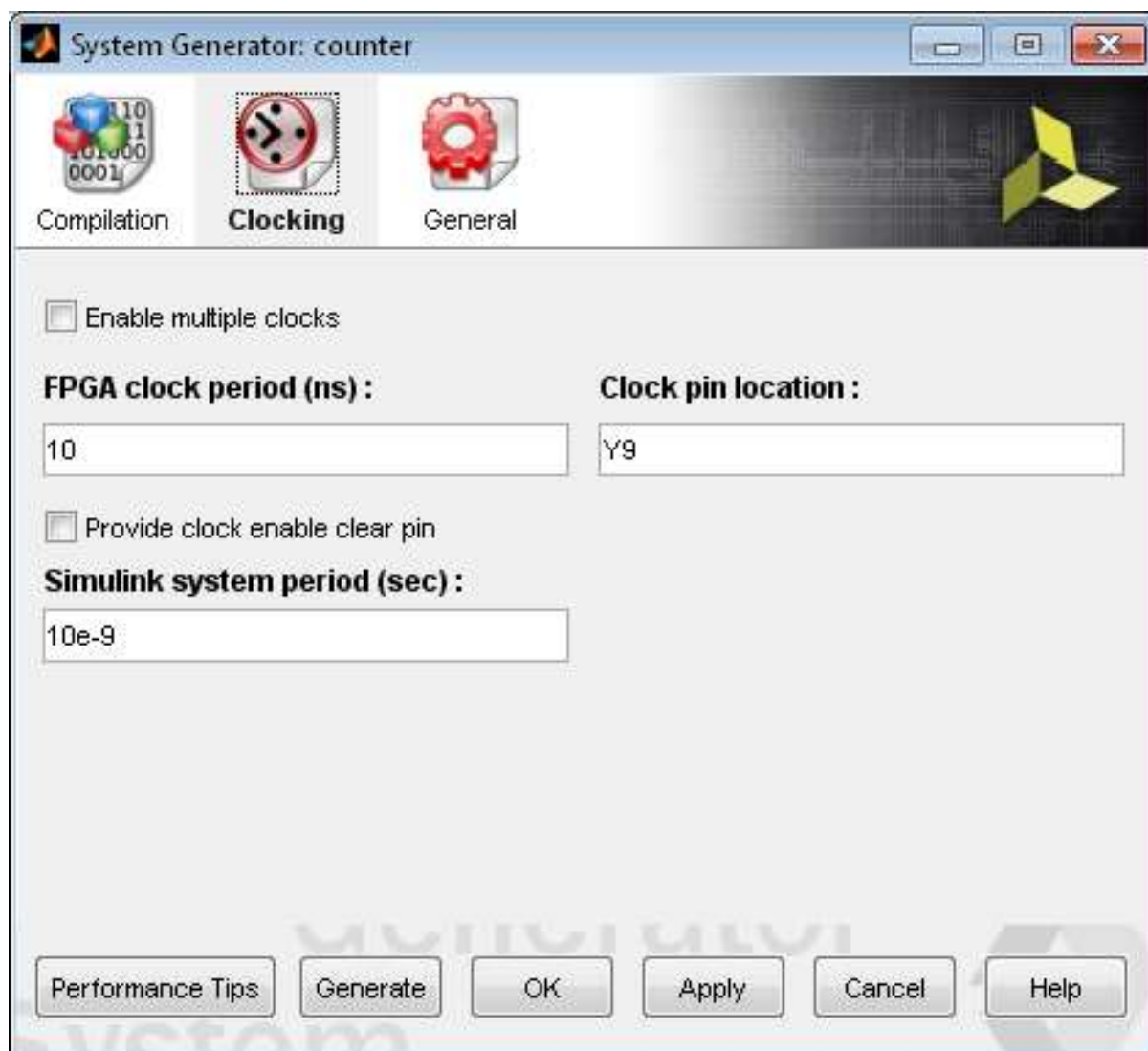
Figure 1.114: System Generator block configuration (2)
