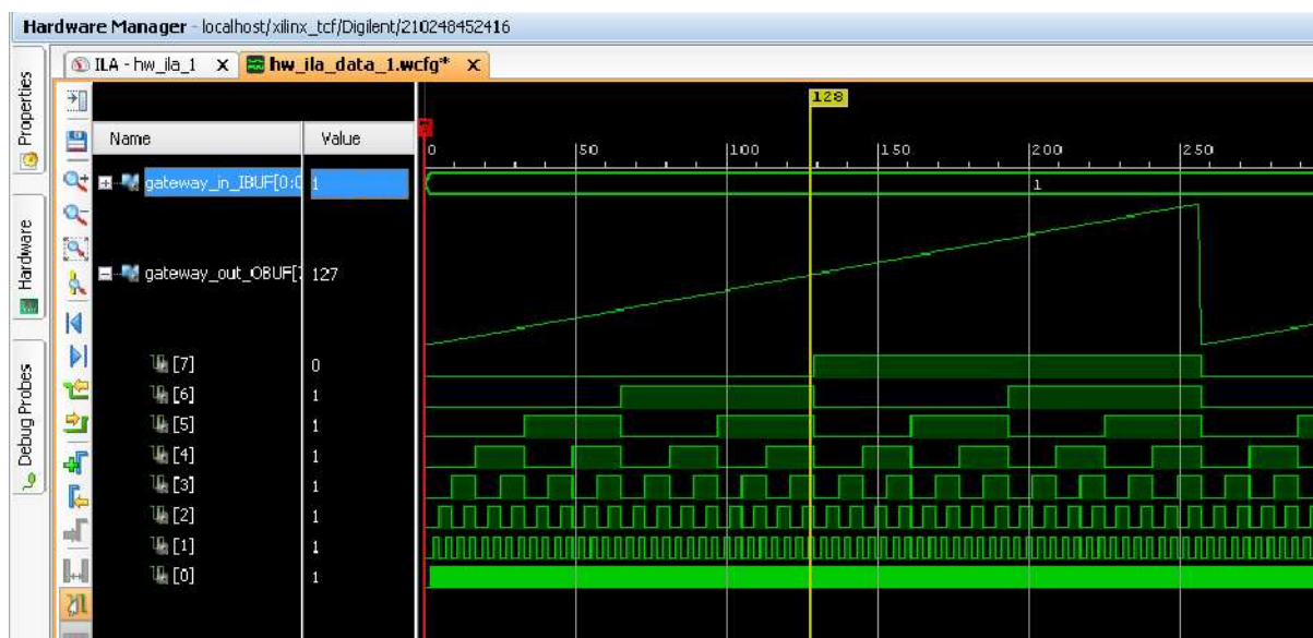
Figure 1.119: Counter output in ILA (real-time)
