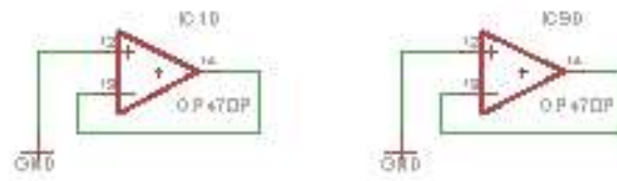
Figure 1.32: Disabling unused op-amps
