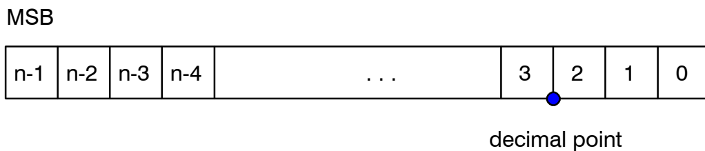
Figure 1.11: Integer with fractional bits (3 bits)
