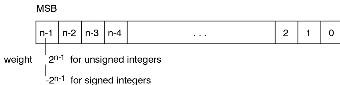
Figure 1.10: Bits of a n bit fixed point number
