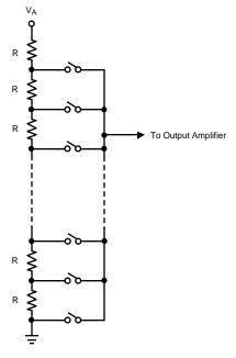
Figure 35. DAC Resistor String
