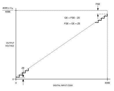
Figure 1. Input / Output Transfer Characteristic
