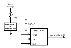
Figure 42. The LM4050 as a power supply
